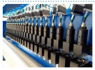
This device OCCUPIES LITTLE SPACE and is designed to punch MACRO HOLES of various diameters and shapes in MOVING MATERIAL and in particular, it works with PLAIN OR PRINTED FILM. This model has to be integrated into existing machinery such as extruders, slitters, bag machines etc. It is suitable to make holes on fruits and vegetables bags, garbage bags, paper bags, foam etc.
